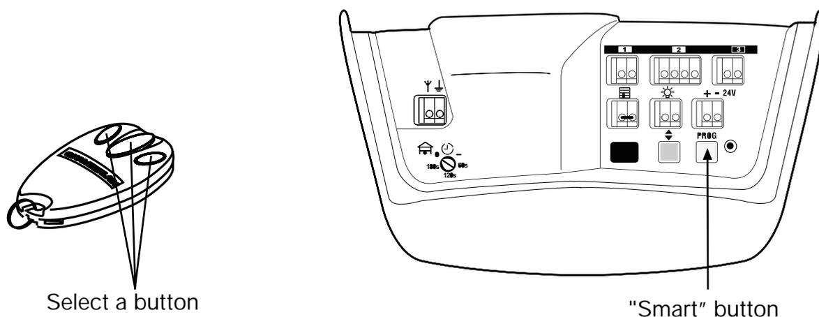
FIGURE 7 Programming the receiver
