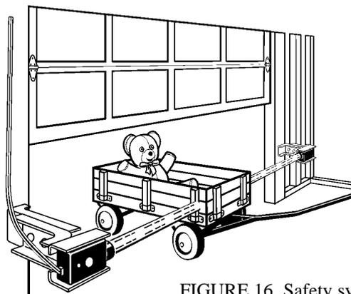
FIGURE 16 Safety system (IR Sensor System)
