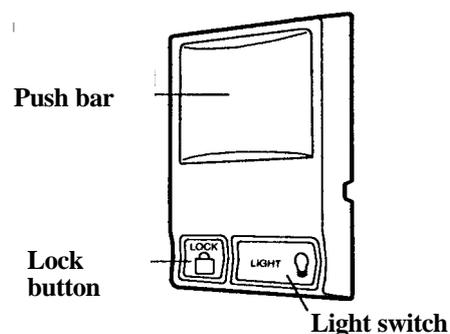
FIGURE 9 Multi-function door control panel
